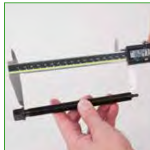
b Measure the thread length to the tip of the spindle
