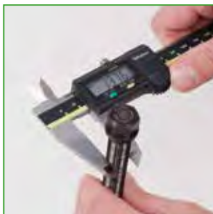
a Measure the spindle diameter.
